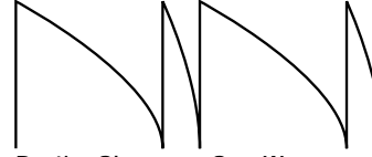
Positive Skew on a Saw Wave
