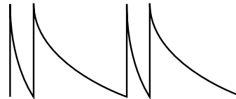
Negative Skew on a Saw Wave
